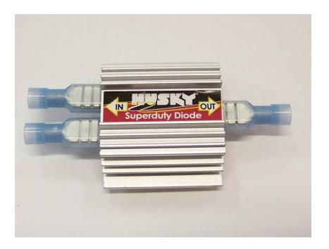
Premium Tail Light Isolator. Provides a safe and convenient way to use factory lights on towed vehicles while protecting sensitive electronics from voltage feedback. Permanently installs on tow vehicle, near tail lights. Heavy duty, 30-amp rating. Aluminum heat sink prevents diode failure caused by overheating. Easy installation: includes connectors and adhesive mounting pad.
