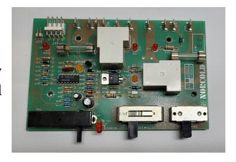
Refrigerator Power Supply Circuit Board; Replacement For Norcold Refrigerator Series 876 EG3\ 878 EG3; 3 Way
