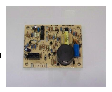
Ignition Control Circuit Board; Replacement For Suburban 520820 Board And Fits All Suburban 12 Volt Furnaces; Will Not Replace 24 Volt AC Boards
