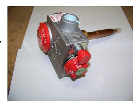
Rv gas water heater thermostat gas control. 160F Max. Model R103RVTLPPA. Has built-in single cycle ECO system. Shank Length 1-1/2". Sensing tube 5-1/2". Inlet 3/8" FPT. Outlet 3/8" FPT.
